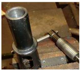
Next - bolt the pieces together and discover just how well you did in aligning the surfaces. You can fix any problems with a bit of care on the grinder or with a file but....
