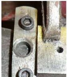
Start with two pieces of steel (here <sup>3</sup>/<sub>4</sub>" x 3/8" x 2.0"). They just have to be thick enough not to bend easily (small angle iron would do), wide enough to drill and tap the bolt holes, and long enough to span the actual blade height plus room for the bolts. The bolts here are 8x32 socket cap screws. I used them because I have a box of a 100. I would not do lighter and anything over <sup>1</sup>/<sub>4</sub> is way overkill.
