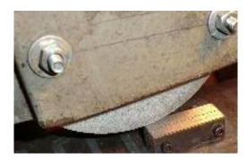
The freshly cut surfaces will almost instantly rust in the humidity typical of Florida. While I could paint the unit, I prefer to use hot bees wax. A cheap heat gun, a loaf pan of wax, tongs to fish the hot metal out of the molten wax makes a pretty good anti-rust system.
