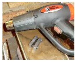
Here is the Alignment Guide ready for use. Note that one corner has been ground down to make an index. I can guarantee that if you don't do this, there will come a time when you will assemble the unit incorrectly. If you are lucky, you will catch the problem before putting a set of bolster on out of alignment.
