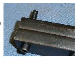
I have a mill (Series 1 Bridgeport clone) with a flood coolant system, so it's over to the mill to run a shallow cut to insure that both the front and back surfaces are precisely aligned.
